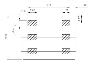
Material: Wire Retention Spring: PhBz, Matte Tin over Ni Plating Insulating Body: LCP, UL94V-0, White Electrical Voltage Rating: 150 VAC Current rating: 3 Amp Wire Range: 22-26 AWG, Solid Wire Strip Length: 5-6mm Withstand Voltage: 1.3KV Mechanical -40°C to +130°C Operating Temperature: -40°F to +266°F 260°C/10 Sec max Reflow Soldering temperature: Safety Approval:
