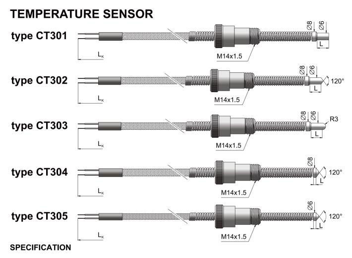
Application temperature measurement of feed cylinders extruding presses
