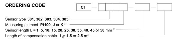
**Example for order**: CT-301J-10-1,5 thermocouple sensor Fe-CuNi (J), length L=10 mm with cable of length  $L_{\rm k}$ = 1.5 m and fitting with thread M14x1.5.
