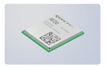
Quectel AF20 is a cost-effective Wi-Fi & BT\* module with high performance. The ultra-compact 17.2mm × 15.2 mm × 2.2mm profile makes it a perfect choice for size sensitive applications. The compact and unified form factor can also help customers reduce product sizes and cut costs.
